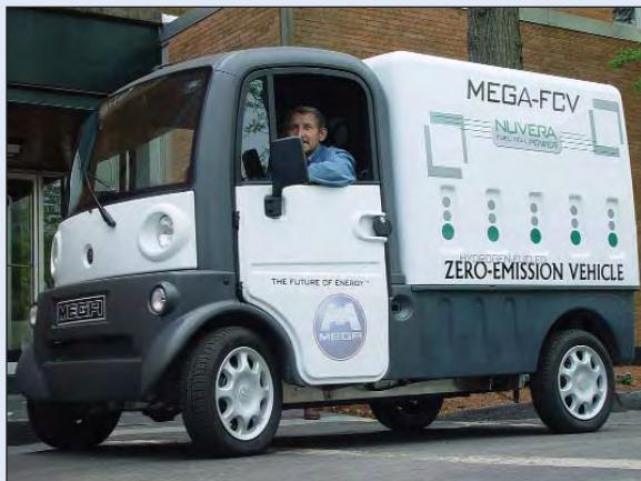
*Fuel cell powered zero emission vehicle.*
